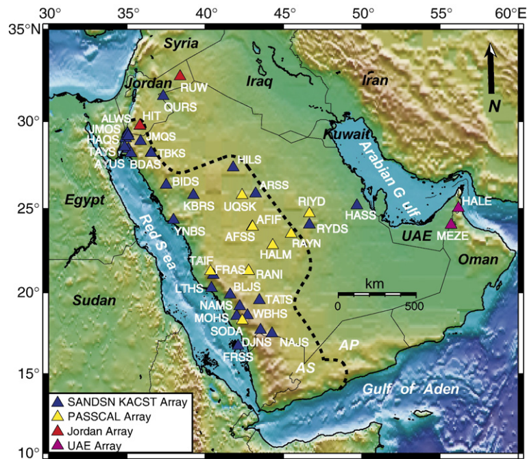
Fig. 2. Station map. The four different colors of triangles indicate the four seismic networks included in this study. SANDSN: blue, IRIS-PASSCAL: yellow, Jordan: red, UAE: pink. The corresponding station names are also listed. The dashed black line shows the boundary between the Arabian Shield (AS) and the Arabian Platform (AP).
